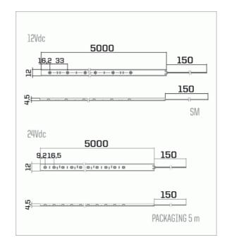
Monochrome LED and RGB light signaling system on flexible strip with double resin protection. Supplied with 3M tape for application on a wide array of surfaces. It is ideal for creating light profiles, effect lighting of niches and glass cabinets. Available in the Warm White, Cold White (12Vdc / 24Vdc) and RGB (24Vdc only) versions.
