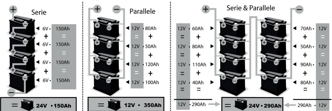
SCHÉMAS ÉLECTRIQUES / CIRCUIT DIAGRAM / SCHALTPLAN / DIAGRAMA ELECTRICO /
