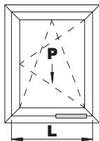
$P < 50 \text{ Kg}$   $364 \text{ mm} \leq L < 800 \text{ mm}$
